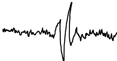
FIG. 3. The (1/2 \leftrightarrow 5/2) pure quadrupole transition (forbidden transition) of Bi 209 in BiCl 3 .
