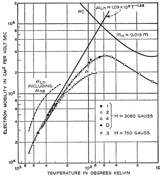
FIG. 6. Electron mobility *vs* temperature.
