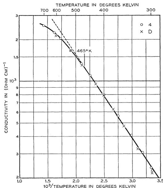
FIG. 5(b). Conductivity vs reciprocal temperature in the intrinsic range.
