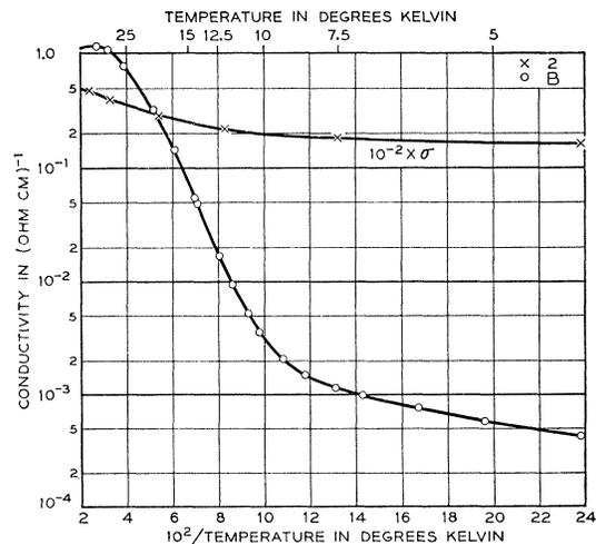
FIG. 3. Conductivity below  $50^\circ\text{K}$  vs reciprocal temperature for Samples 2 and B.
