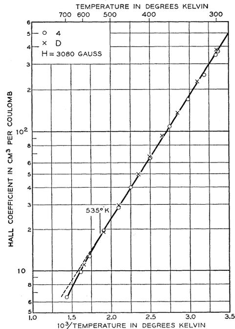
FIG. 4(b). Hall coefficient vs reciprocal temperature in the intrinsic range.
