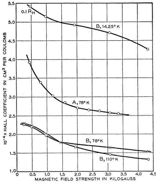
FIG. 1. Variation of Hall coefficient with magnetic field for *p*-type InSb.
