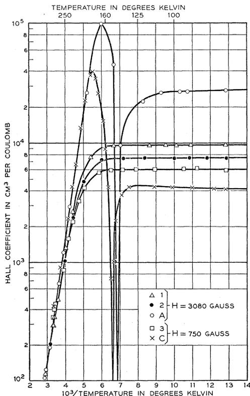
FIG. 4(a). Hall coefficient vs reciprocal temperature from 78°K to room temperature.
