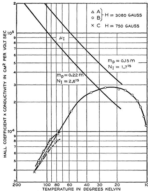
FIG. 7. Hole "mobility" *vs* temperature.
