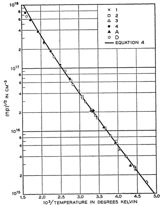
FIG. 8. Square root of the product of electron and hole concentration *vs* reciprocal temperature in the intrinsic range.
