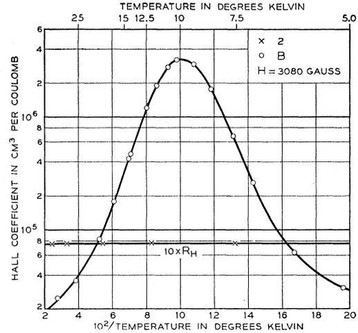
FIG. 2. Hall coefficient below  $50^\circ\text{K}$  vs reciprocal temperature for Samples 2 and B.
