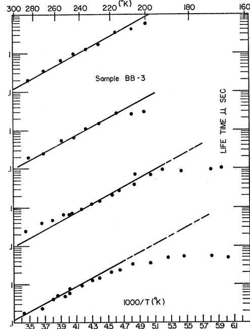
FIG. 3. Electron lifetime as a function of temperature for the high-resistivity  $p$ -type nickel-doped germanium sample for which Hall coefficient and resistivity data are shown in Fig. 2.
