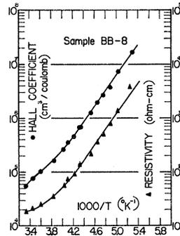
FIG. 1. Resistivity and Hall coefficient as a function of temperature for a high-resistivity  $n$ -type nickel-doped germanium sample.
