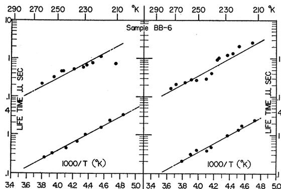
FIG. 5. Electron lifetime as a function of temperature for the high-resistivity *p*-type nickel-doped germanium sample for which resistivity and Hall coefficient data are shown in Fig. 4.
