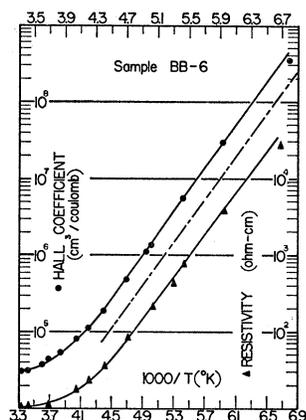
FIG. 4. Resistivity and Hall coefficient as a function of temperature for a high-resistivity *p*-type nickel-doped germanium sample which presumably also contains a small amount of copper. The broken line indicates the theoretically calculated slope of the carrier concentration for a sample that contains  $1.0 \times 10^{15}$  group V donors,  $1.1 \times 10^{15}$  nickel atoms, and  $1.1 \times 10^{14}$  copper atoms per  $\text{cm}^3$ .
