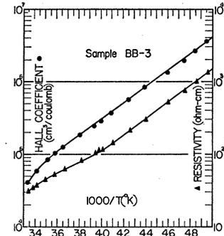
FIG. 2. Resistivity and Hall coefficient as a function of temperature for a high-resistivity  $p$ -type nickel-doped germanium sample.
