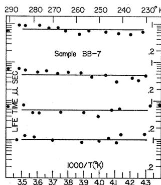
FIG. 6. Electron lifetime as a function of temperature for a low-resistivity *p*-type nickel-doped germanium sample.
