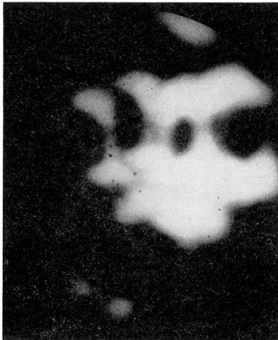
FIG. 2. Typical field emission pattern from titanium crystal that has not been heated above its transformation temperature. Pattern shows no long-range symmetry.
