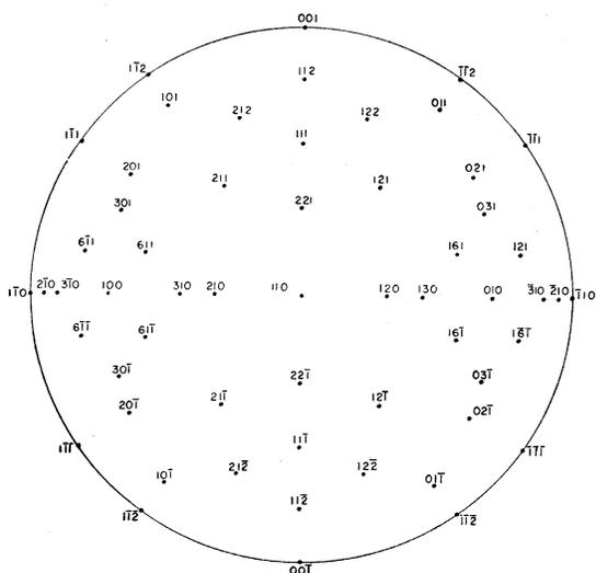
FIG. 8. (110) orthographic projection of poles of some major crystallographic planes of the body-centered-cubic phase in titanium.
