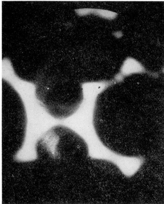
FIG. 4. High-temperature field emission pattern from titanium showing cubic symmetry.
