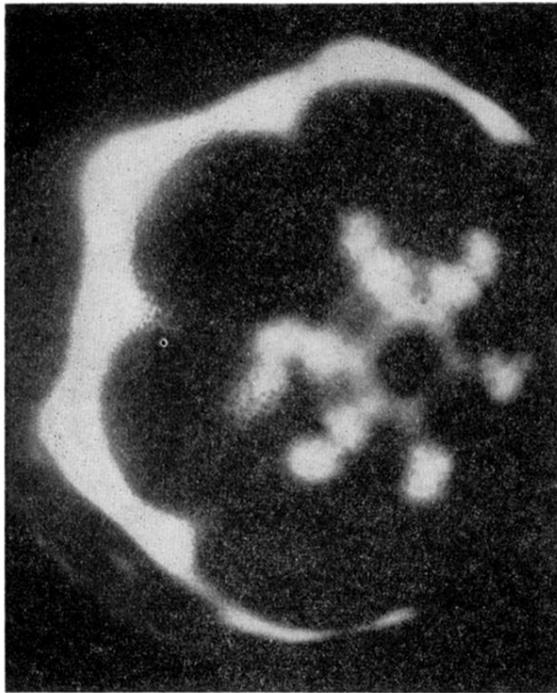
FIG. 14. Field emission pattern from crystal that gave the patterns in Figs. 6(a) through 6(e) taken after crystal was returned from high temperature to room temperature. The original orientation and single crystal are preserved.
