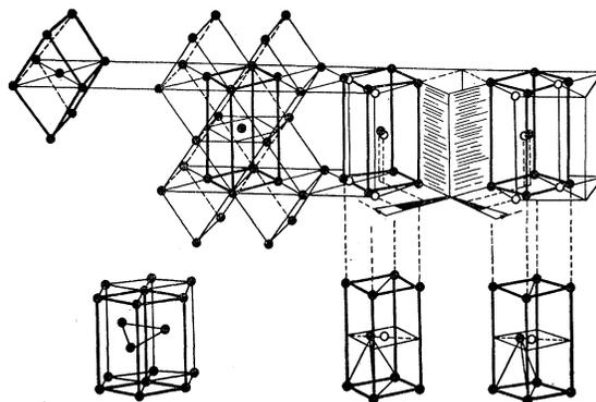
Fig. 12. Burgers' transformation scheme for titanium produces the required orientation relation between high-temperature body-centered-cubic beta phase and low-temperature hexagonal-close-packed alpha phase.
