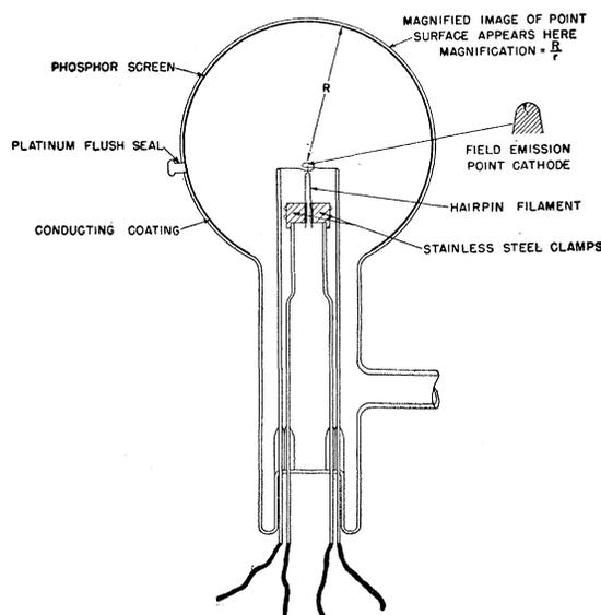
Fig. 1. Experimental field emission microscope in which the effect of phase transformations on the field emission patterns from titanium microcrystals is observed.
