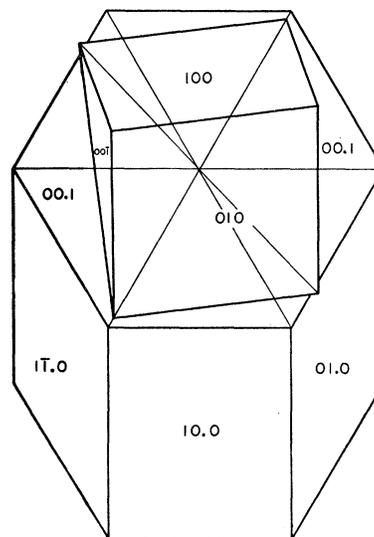
Fig. 13. Illustration of the orientation relation shown in Fig. 11 between the cubic and hexagonal phases of the titanium crystal that gave the series of field emission patterns Figs. 6(a) through 6(e).
