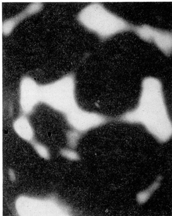
FIG. 3. Field emission pattern from titanium crystal that has been heated above its transformation temperature. Long-range hexagonal symmetry is discernible but imperfect.
