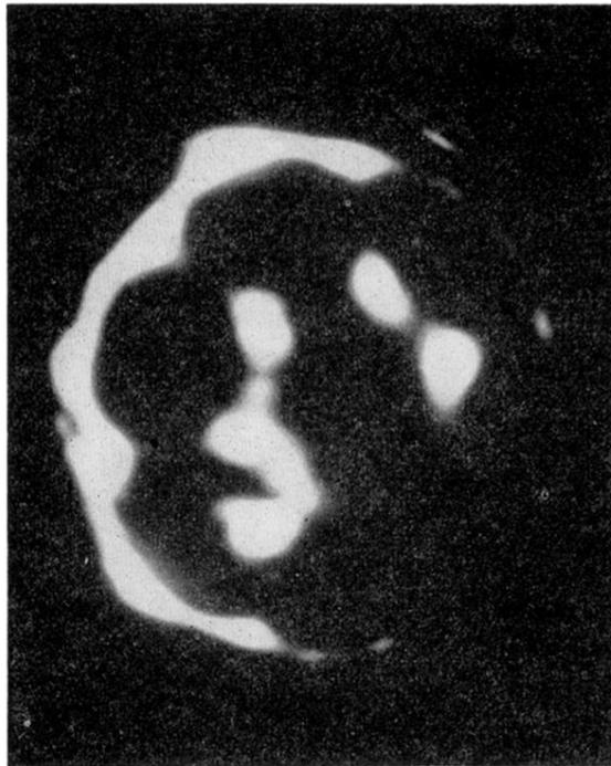
FIG. 5. Low-temperature field emission pattern from a titanium crystal that has been cooled in the presence of an electric field.
