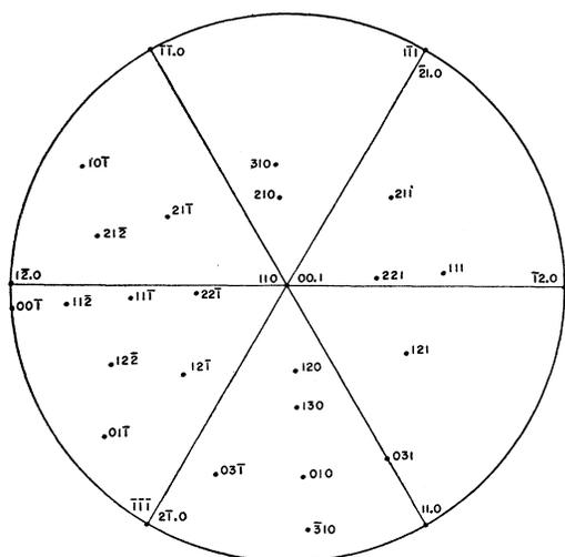
Fig. 11. Composite plot of the poles of the major crystallographic planes of the body-centered-cubic pattern identified in Fig. 10 with the trigonal axes found for the hexagonal-close-packed pattern of Fig. 9. The Burgers orientation relation is obeyed.
