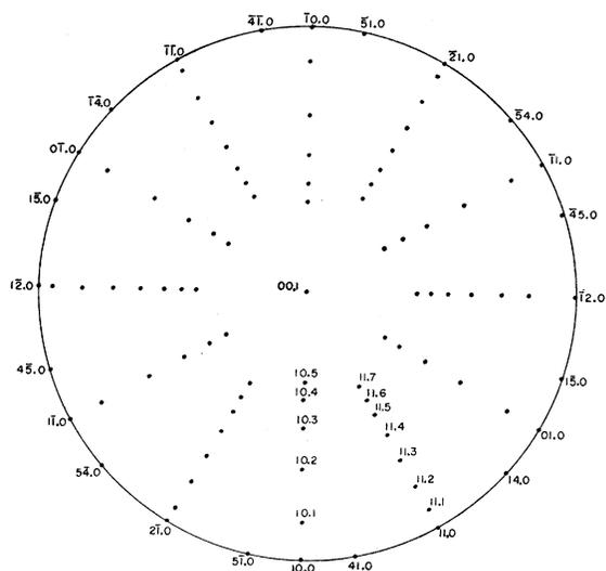
FIG. 7. (00·1) orthographic projection of poles of some major crystallographic planes of the hexagonal-close-packed phase in titanium.  $c/a=1.587$ .
