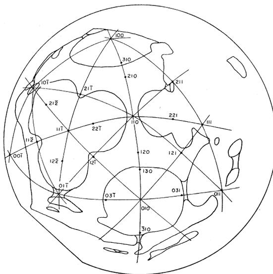
FIG. 10. Location of major crystallographic planes and zones of Fig. 6(e).
