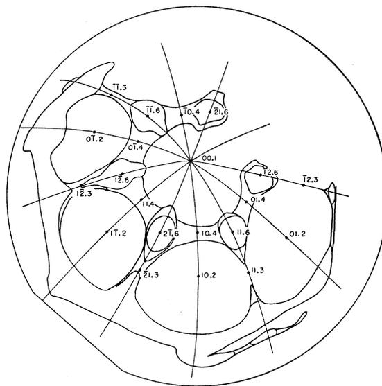
FIG. 9. Location of major crystallographic planes and zones of Fig. 6(a).
