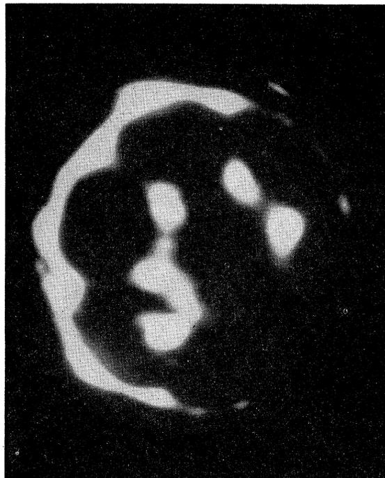
FIG. 5. Low-temperature field emission pattern from a titanium crystal that has been cooled in the presence of an electric field.
