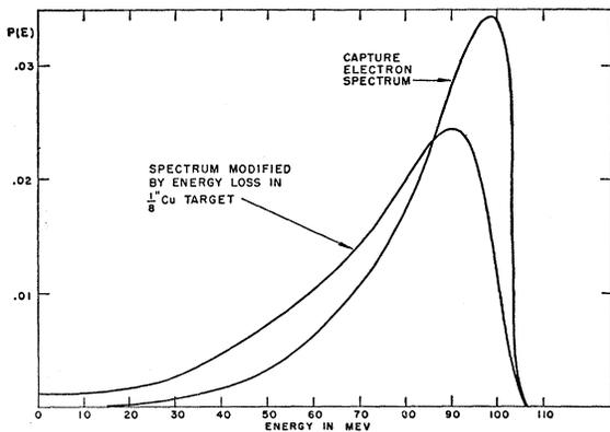
FIG. 2. The spectra of capture electrons calculated on the basis of the Chew-Goldberger model, with and without energy losses in the Cu target.
