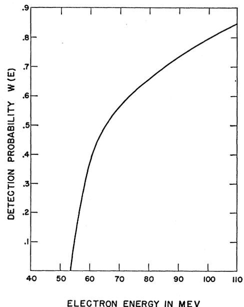
FIG. 3. Detection probability for electron detector with 21 g/cm<sup>2</sup> of polyethylene absorber added.
