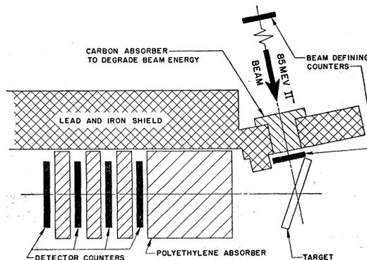
FIG. 1. Experimental arrangement.
