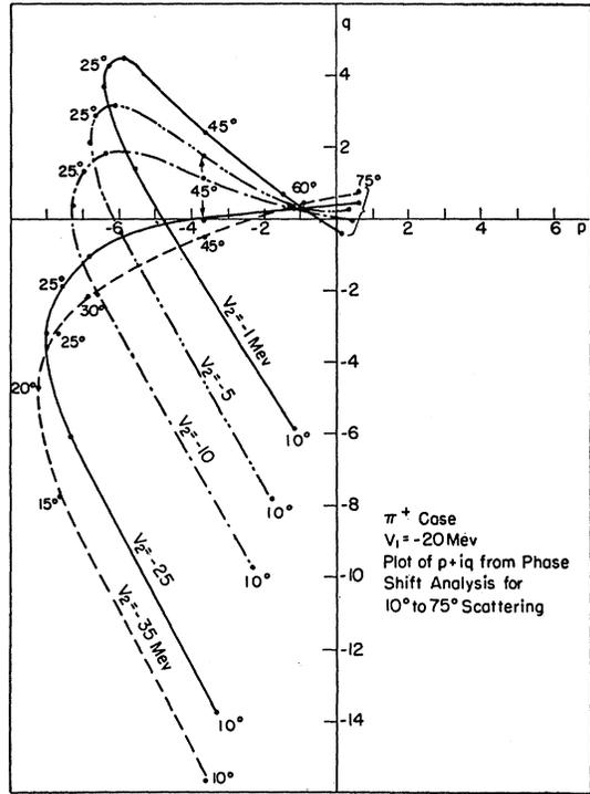
FIG. 9. Plot of  $p+iq$  for  $\pi^+$  mesons from phase-shift analysis for  $10^\circ$  to  $75^\circ$  scattering.
