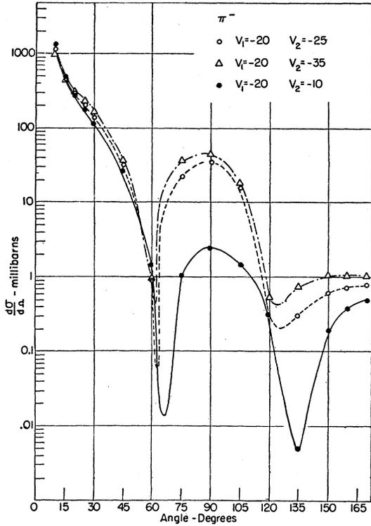
FIG. 5. Differential cross section for 79-Mev  $\pi^-$  mesons on aluminum calculated using phase-shift analysis on optical model for the nucleus, for  $V_1 = -20$  Mev,  $V_2 = -10, -25, -35$  Mev. Plotted points correspond to calculated points.
