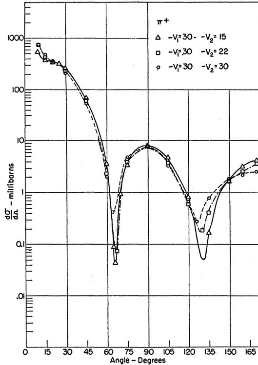
FIG. 1. Differential cross section for 79-Mev  $\pi^+$  mesons on aluminum calculated using phase-shift analysis on optical model for the nucleus, for  $V_1 = -30$  Mev,  $V_2 = -15, -22, -30$  Mev. Plotted points correspond to calculated points.
