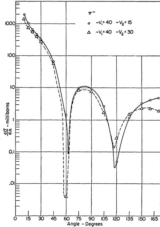
FIG. 6. Differential cross section for 79-Mev  $\pi^-$  mesons on aluminum calculated using phase-shift analysis on optical model for the nucleus, for  $V_1 = -40$  Mev,  $V_2 = -15, -30$  Mev. Plotted points correspond to calculated points.
