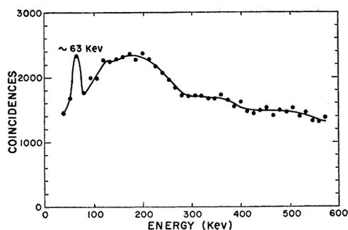
FIG. 3. Partial spontaneous fission fragment gamma-ray coincidence spectrum of  $\text{Cf}^{250,252}$ .
