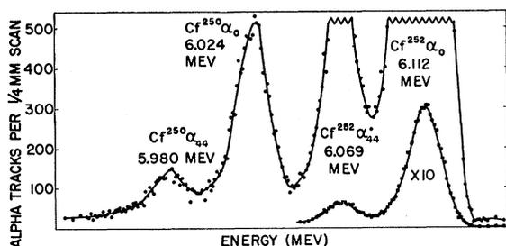
FIG. 1. Alpha spectra of  $\text{Cf}^{250}$  and  $\text{Cf}^{252}$ .
