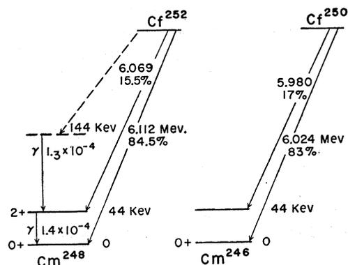
FIG. 4. Alpha-decay schemes of  $\text{Cf}^{250}$  and  $\text{Cf}^{252}$ .
