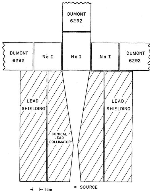
FIG. 1. Geometry of the three-crystal pair spectrometer.
