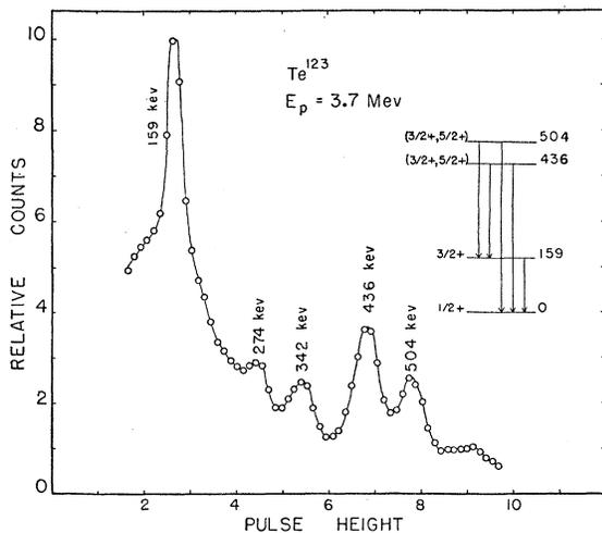
FIG. 1. Pulse-height spectrum from  $\text{Te}^{123}$  bombarded with 3.7-Mev protons.
