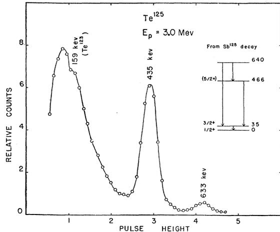
FIG. 2. Pulse-height spectrum from  $\text{Te}^{125}$  bombarded with 3.0-Mev protons. The broad peak at the low-energy end is due to proton bremsstrahlung. The small hump in this peak at 159 keV is due to a slight contamination of  $\text{Te}^{123}$ .
