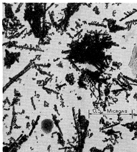
FIG. 3. Fine particle iron C. Median elongation 3.0; coercive force 1600 oersteds.
