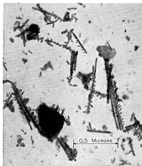
FIG. 6. Fine particle iron E . Median elongation 4.6; coercive force 1850 oersteds.
