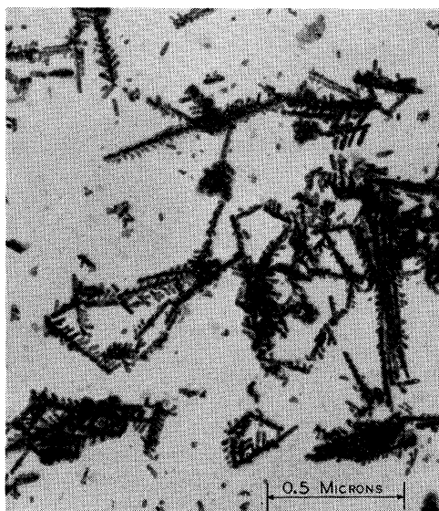
FIG. 4. Fine particle iron D . Median elongation 4.0; coercive force 1600 oersteds
