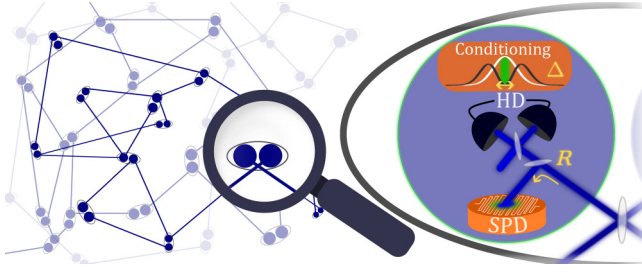
FIG. 1. A sketch of the hybrid Bell-state measurement (HBSM), consisting of on-off single-photon detection (SPD) and quadrature conditioning via homodyne detection (HD) in a network configuration. At a network node, two optical modes are mixed on a balanced beam splitter. One of the output modes is tapped via a beam splitter with reflectivity R and this part is sent to an SPD. The transmitted mode is directed to a HD, which is used for conditioning on quadrature values in a window \Delta around q = 0 . The HBSM success is heralded by both detection events.
