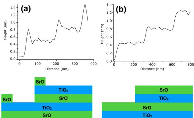
FIG. 2. AFM line profiles perpendicular to step edges. (a) Line profile of a surface that has been treated such that SrO is segregated to the step edges. (b) Line profile of a surface that has been treated to obtain SrO termination. Bottom figures illustrate the distribution of SrO and TiO<sub>2</sub> planes corresponding to the line profiles.
