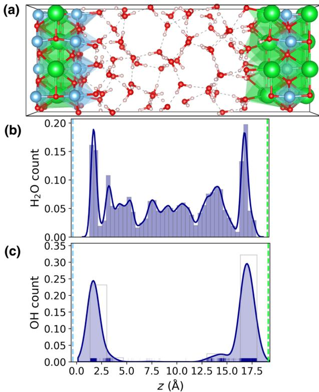
FIG. 4. An equilibrated molecular dynamics simulation for (a) (001) SrTiO<sub>3</sub> surfaces—TiO<sub>2</sub> (left, in blue) and SrO (right, in green)—interacting with a box of 64 water molecules. The number density distribution along the vertical  $z$  direction for (b) H<sub>2</sub>O molecules and (c) dissociated OH<sup>-</sup> species. The positions of the TiO<sub>2</sub> and SrO surfaces with respect to the box of water are shown with blue and green dashed lines, respectively.
