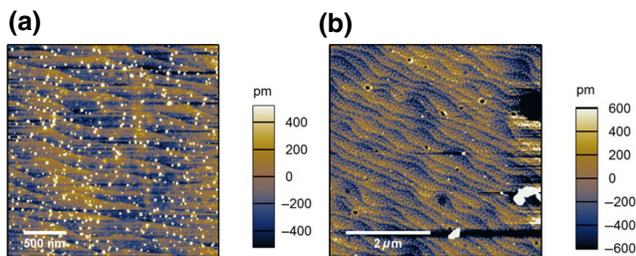
FIG. 3. AFM topography scans of  $\text{TiO}_2$ -terminated surfaces after silver deposition on (a) a treated substrate and (b) a deposited  $\text{SrTiO}_3$  film.
