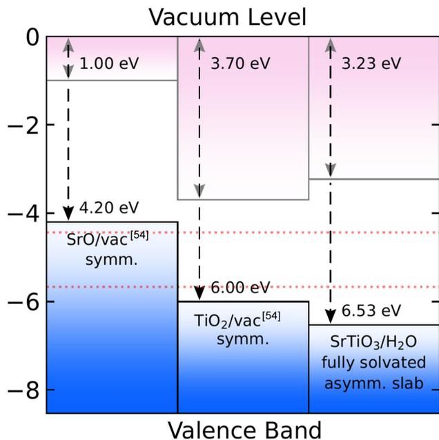
FIG. 5. Band alignments for symmetric SrO-terminated and symmetric TiO<sub>2</sub>-terminated SrTiO<sub>3</sub>/vacuum as reported in Ref. [54], and fully solvated SrTiO<sub>3</sub>/H<sub>2</sub>O slabs using DFT HSE06. The red dotted lines indicate the water redox potentials referenced to the vacuum level ( $E_{\text{H}^+/\text{H}_2} = -4.44$  eV,  $E_{\text{O}_2/\text{H}_2\text{O}} = -5.67$  eV).
